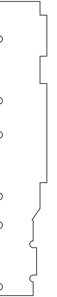
Edge Rib Make 4 - .125 thick
