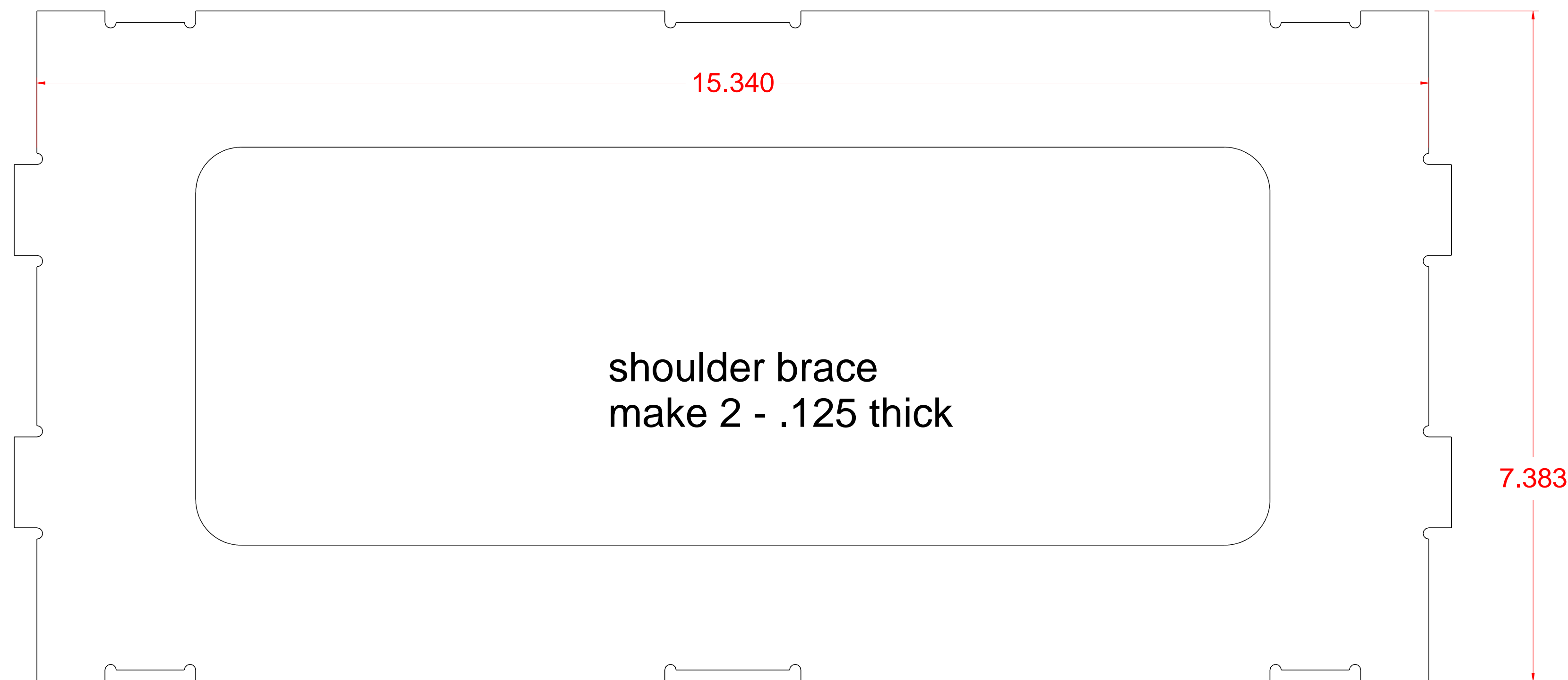
shoulder plate make 2 - .25 thick or - make 4 - .125 thick
